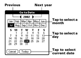
**Tip:** In the Go to Date dialog box, you can also use the scroll buttons on the front panel of your handheld to move forward or backward one month at a time.
