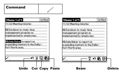
The command toolbar displays context sensitive menu commands for the current screen. For example, if text is selected the menu icons displayed may be undo, cut, copy, and paste. Tap on an icon to select the command, or immediately write the corresponding command letter for an appropriate command in the Graffiti writing area.
