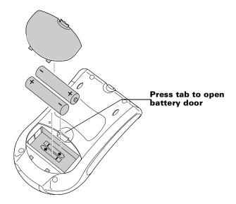
2. Install the two AAA alkaline batteries supplied with your handheld into the battery compartment.
