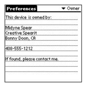
If you assign a password with the Security application, the information in the Owner Preferences screen cannot be changed. In this case, an Unlock button appears at the bottom of the screen.
