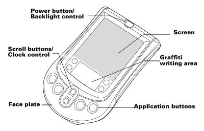
Power button/ Backlight control Turns your handheld on or off and controls the backlight feature. If your handheld is turned off, pressing the power button turns the unit on and returns you to the last screen you viewed.
