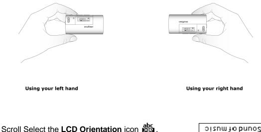
The LCD screen rotates 180 degrees (Figure 3-46).
