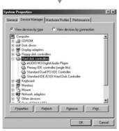
Finally, make sure that installation of iAUDIO M3 was completed normally by checking "iAUDIO M3 Digital Audio Player" displayed under Control Panel →System →Device Manager → Hard Disk Controller.
