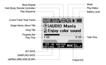
The battery level icon indicates how much battery life is left. The number of segments in the icon becomes less as the battery discharges. For some batteries or re-chargeable dry cells, the number of segments in the battery icon may increase or decrease irregularly when the remaining charge is being measured. This is normal.
