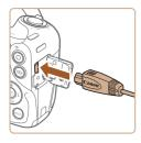
On the camera, open the terminal cover and insert the cable plug fully into the camera terminal.
