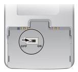
**CAUTION:** Always leave the backup battery switch in the ON position for normal operation. Changing the switch will cause your data to be lost.
