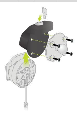
2. Lock your TomTom Rider to prevent removal from the mount. Unscrew the wingnut from the RAM arm and attach the RAM lock.
