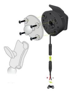
Important: The red POS (+) contact needs to be connected to the motorcycle's wiring loom at a point between the ignition and the +12V battery supply. The black NEG (-) wire needs to be connected to the motorcycle's wiring loom at a point between the ignition and the -(GND) battery supply. Attach to a 12V point that can be switched off by the ignition such as the light circuit.
