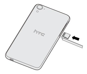
**3.** To close the slot cover, slightly move it side to side to let the rubber hinge sink down by itself. Then gently press down the cover.
