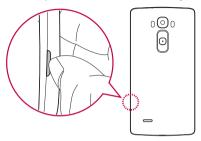
2 Slide the SIM card into the lower slot for the SIM card as shown in the figure. Make sure the gold contact area on the card is facing downward.
