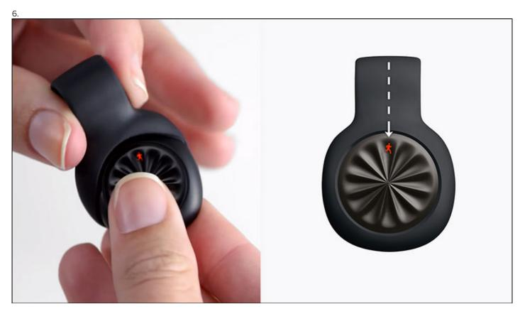
Place the tracker back into the clip with the runner icon at the top in the 12 o'clock position.
