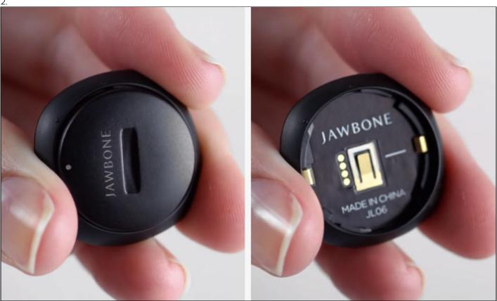
Use the battery tool to twist the cap counter-clockwise until the battery cap comes off.
