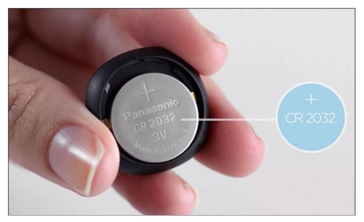
Insert a CR2032 battery with the "+" facing outwards.
