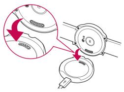
3 Plug the small end of the USB cable provided into the charging cradle's USB port.
