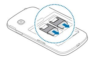
► Single SIM models: Pull out the SIM or USIM card.
