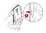
To remove the back cover, hold the phone firmly in one hand. With your other hand, lift off the back cover with your thumbnail as shown in figure below.
