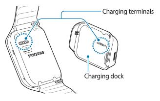
2. Place the Gear™ 2 Neo on the charging dock with the charging terminals facing each other.
