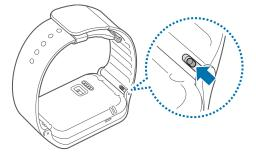
2. Lift the strap out to detach it from the Gear™ 2 Neo.
