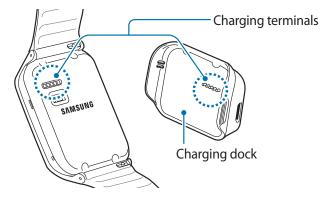
2. Place the Gear on the charging dock with the charging terminals facing each other.
