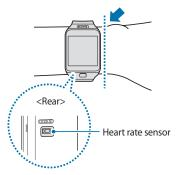
Important! Remove the protective plastic from the heart rate measurement sensor before taking measurements.
