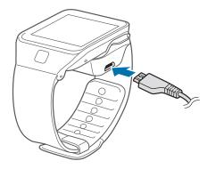
4. After fully charging, disconnect the Gear 2<sup>™</sup> from the charging dock.
