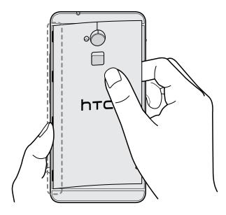
2. Close the back cover and press starting from the top to the bottom. Make sure that there are no gaps on any side.
