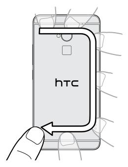
**3**. Press again on the right side to secure the cover into place, and then slide the lock all the way to the closed position.
