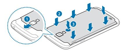
To avoid water damage, ensure that the back cover is completely closed by pressing just below the flash (3) until you hear a click.
