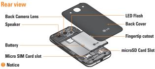
The NFC antenna for this model is on the back cover.
