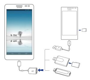
To connect your phone to another phone, make sure that the phone you wish to connect to supports the USB mass storage function and has a microSD card installed. To establish the connection and read data stored on the microSD card:
