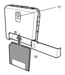
16 Insert SMC card in the correct direction, as shown.
