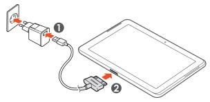
Connecting the USB cable improperly may cause serious damage to the device or USB power adapter. Any damage caused by misuse is not covered by the warranty.
