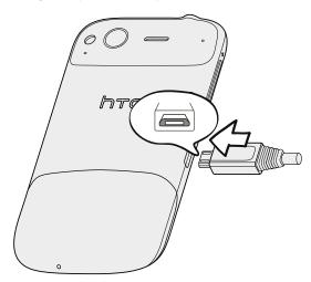
2. Plug in the power adapter to an electrical outlet to start charging the battery.
