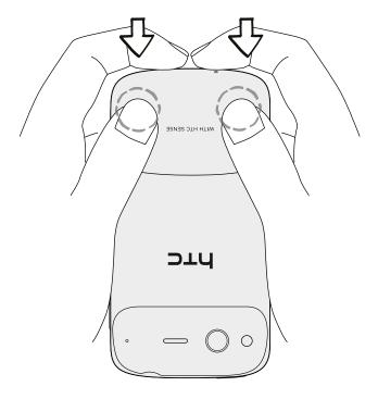
Your phone's antenna is placed underneath the bottom cover. We recommend that you make sure the bottom cover is correctly secured to the phone's back panel to get the best radio reception for your phone.
