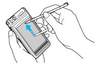
To drag, press the stylus lightly on the item and move it along the screen surface to its new position.
