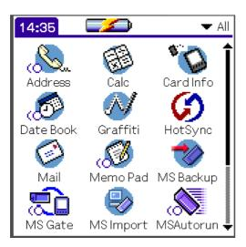
As well as being your gateway to all the applications, the **Application Launcher** screen displays the current time, battery level, and application category.
