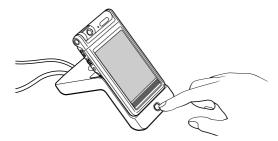
When the HotSync<sup>®</sup> operation is complete, a message is displayed on your CLIÉ handheld. Do not remove your CLIÉ handheld from the cradle until the HotSync<sup>®</sup> operation is complete. Otherwise the Palm<sup>TM</sup> Desktop for CLIÉ software may not quit normally and you may have to perform a soft reset.
