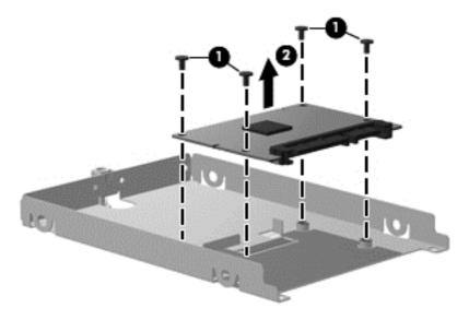
Reverse this procedure to install a hard drive or solid state drive.
