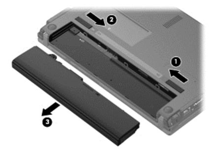
Reverse this procedure to install a battery.
