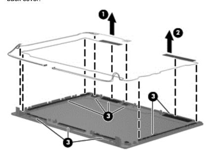
b. Remove the wireless antennas and cables.
