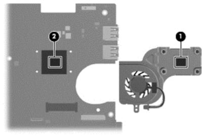
Reverse this procedure to install the fan and heat sink assembly.
