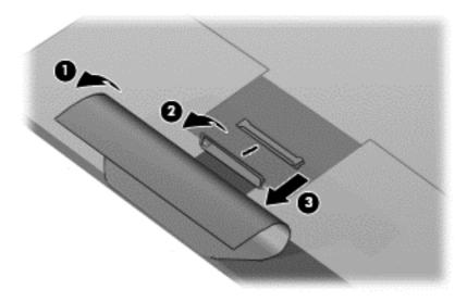
**c.** Release the display panel/webcam cable **(1)** from the adhesive points **(2)** along the cable route on the back of the display panel.
