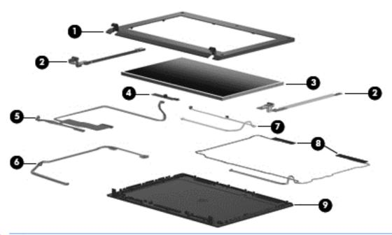
NOTE: The following figure shows the components of the touch-screen display assembly. The display bezel thickness increases to accommodate the touch-screen glass and board.
