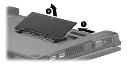
3. Spread the retaining tabs (1) on each side of the memory module slot to release the memory module. (The module tilts up.)
