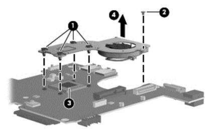
NOTE: The thermal material must be thoroughly cleaned from the surfaces of the fan and heat sink assembly and the system board each time the fan and heat sink assembly is removed. Thermal paste is used on the processor (1). Replacement thermal material is included with all fan and heat sink assembly, and system board spare part kits.
