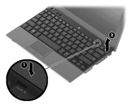
Use your right hand to lift up (1) and remove the retention tab from the middle of the top cover **(2)**.
