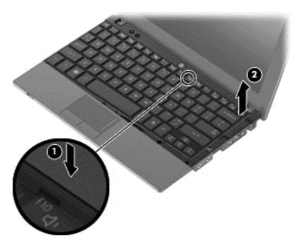
8. Use your left hand to lift up (1) and remove the retention tab from the left side of the top cover (2)..
