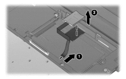
Reverse this procedure to install the SIM module.
