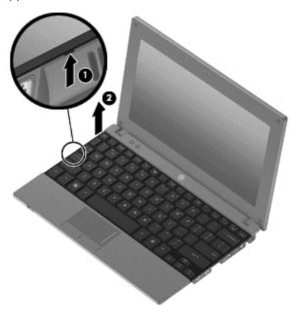
5. Release the retention tab (1) on the right side of the keyboard (2).
