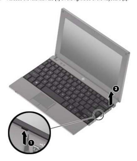
Use your right hand to lift up (1) and remove the retention tab from the right side of the top cover (2).
