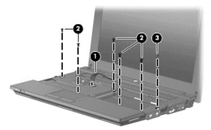
8. Release the clips along the front edge of the top cover and open the front of the top cover (1) enough to see the TouchPad and speaker cables.
