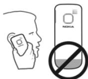
The figure shows the GSM antenna area marked in grey.
