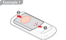
To remove the back cover, press down on the center of the cover and slide it in the direction of the arrow.
