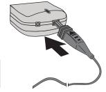
Connect the charger to the mains power supply. The LED on the phone lights to indicate that external power is applied.
