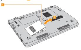
**6** Unlock the card holder **1**, lift it up **2** and then insert the SIM card firmly into the card holder **3**.
