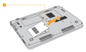
**6** Unlock the card holder **1**, lift it up **2** and then remove the SIM card from the card holder **3**.
