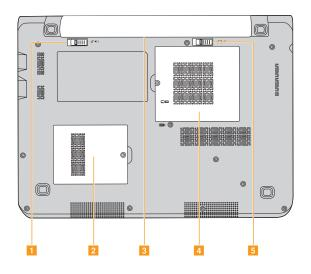
Battery latch spring loaded The spring-loaded battery latch keeps the battery pack secured in place.
