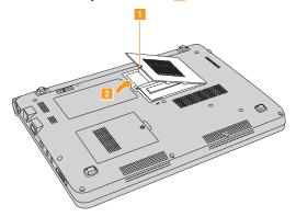
Press outwards on the latches on both edges of the socket at the same time, remove the SO-DIMM. Be sure to save the old SO-DIMM for future use.
