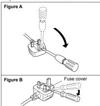
Replace the fuse and close or attach the fuse cover.
