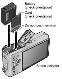
Set the camera ON/OFF switch to OFF Slide to the 'OPEN' position and open the lid
