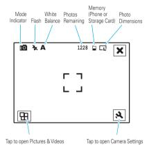
To focus the picture, hold the camera key halfway in until the autofocus box turns green.
