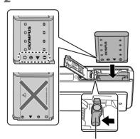
Insert the battery from the ▼ end, with the symbol facing toward the battery lock knob. If the battery is not inserted correctly.
