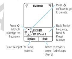
To **adjust radio volume**: Press the volume keys on the side of your phone.
