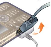
Remove the charger by tilting the plug upwards.
