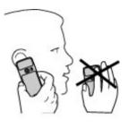
otherwise needed. To optimize antenna performance and battery life, avoid contact with the antenna area when operating the device.
