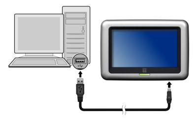
The charge indicator glows amber when charging is in progress. Do not disconnect your device until the battery is fully charged, when the charge indicator turns green. This will take a couple of hours.
