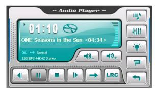
The information area displays the current status such as play/pause/stop status, the elapsed time, the power status, the playback mode, the filename, and the volume level.
