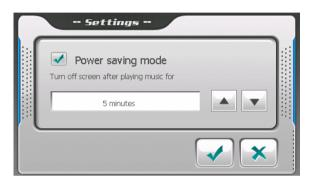
Tap the check box  $(\sqrt{})$  to turn on the power saving mode. Tap the up/down button to set the timer to 10 seconds, 30 seconds, 1 minute, or 5 minutes. During the playback, the screen backlight will automatically shut off if you haven't tapped the screen within the preset time (5 minutes by default). The backlight will restore when you press the power or **Menu** button or when the playback of the current play list has ended.
