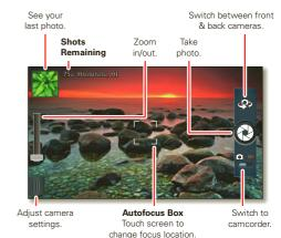
**Note:** Photos are stored in your smartphone's internal memory, unless you switch it to a microSD memory card. Photo resolution can be set to 8MP or **Widescreen** (6MP).
