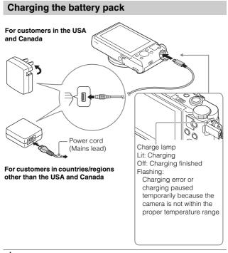
1 Connect the camera to the AC Adaptor (supplied), using the micro USB cable (supplied).
