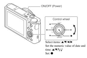
Press the ON/OFF (Power) button. Language setting screen is displayed when you turn on the camera for the first time.
