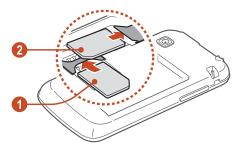
The SIM card slot of your device is only suited for standard SIM cards. Inserting a microSIM card or a microSIM card with an unauthorised holder may cause damage to the SIM card slot of your device.
