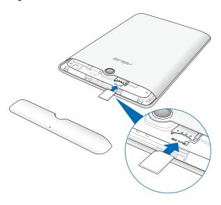
3. Replace the back compartment cover securely in place.
