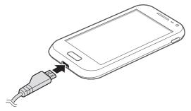
Connecting the travel adapter improperly may cause serious damage to the device. Any damage caused by misuse is not covered by the warranty.
