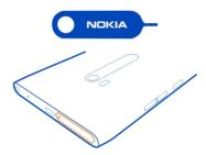
1 Push the SIM door key into the hole in the SIM door until the SIM tray is released, then pull the tray out.
