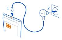
To avoid breaking the USB cable connector, be careful when connecting or disconnecting the charger cable.
