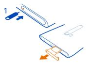
2 Make sure the contact area is facing up, then put the SIM card in the SIM tray.
