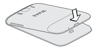
3. Press the back cover down to lock it into place. You'll hear a click when the back cover is locked in place.
