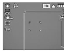
**Remaining battery** (only when using battery)
