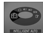
The current mode will be displayed on the LCD monitor when the mode dial is turned.
