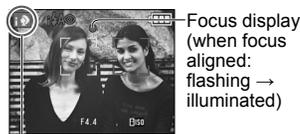
Focus display (when focus aligned: flashing → illuminated)
