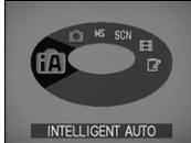
The current mode will be displayed on the LCD monitor when the mode dial is turned.
