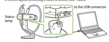
Charging starts. The status lamp blinks slowly during charging. When charging is completed, the status lamp will stop blinking and light dimly while the player is connected to the computer. For details about charging time and the battery duration, see F "Specifications" on the reverse side.
