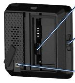
microSD card slot under the battery
