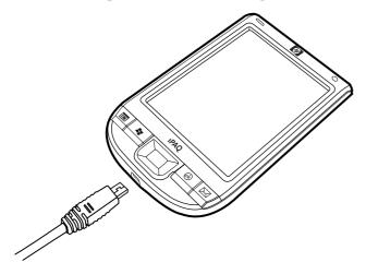
△ CAUTION: To avoid damaging your HP iPAQ or the AC adapter, make sure all connectors are properly aligned before connecting.
