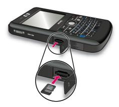
3. Push the card in the slot to lock it in place.
