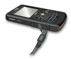
△ **CAUTION:** To avoid damaging your HP iPAQ or the AC adapter, make sure all metal connectors are properly aligned before connecting.
